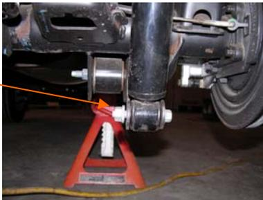
38. Disconnect the lower sway bar end link nut with a 16mm wrench.
