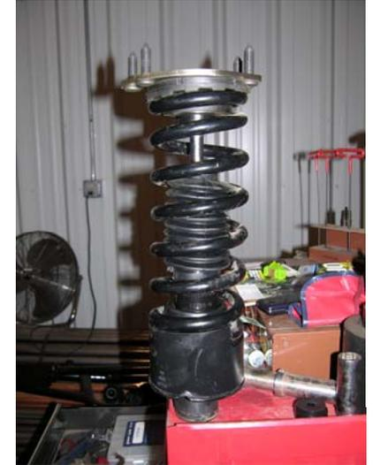
31. Reinstall the strut assembly into the vehicle and start the upper nuts, hand tighten only. Reinstall the lower strut clevis and hand tighten the bolt at the strut. Install the lower clevis bolt into the lower control arm.
