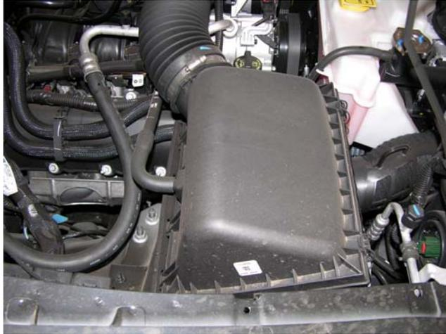
43. Reinstall the TIPM and battery on the left side of the vehicle by following steps, 4 to 12 . Working in reverse order.
