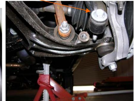
19. Remove the lower bolt at the lower control arm securing the clevis bracket with a 24mm socket.
