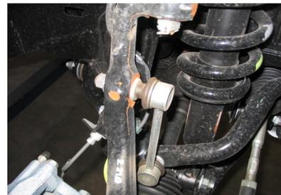
6. Remove the upper strut nuts.( 14mm nuts ) You will need to reuse them later.
