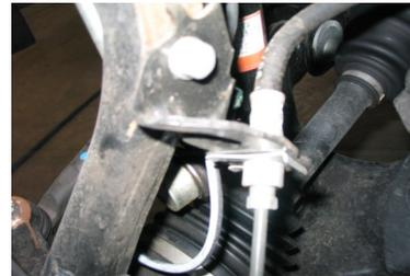
5. Disconnect the sway bar on both side at the spindle. ( 17mm bolt. )
