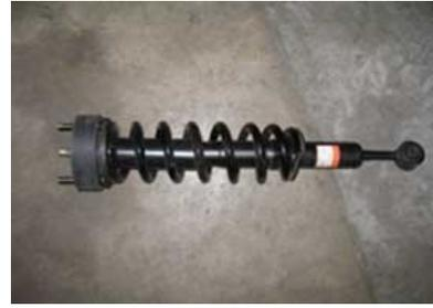
11. Reinstall the strut into the vehicle and tighten the upper strut nuts. You will have to push up on the upper a-arm to get the strut back in.
