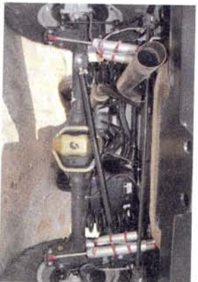
▲ Daystar JK arms are adjustable so we can adjust for caster and lift height. J.E. Reel CV driveshafts are strong and perfectly balanced. There are no driveline vibrations in either Jeep. The front Dana 44 on the JK is reverse-cut with the pinion up high out of harm's way. The front 44s have 30-spline inner axles, but 32-spline outers with big U-joints. Burnsville had the axles machined so full-circle C-clips could be used. The only problem with the JK is that the half-circle C-clips work their way out, letting the U-joint cap fall out. With the U-joint rattling around in the ears, the axle breaks. We had no problems at all with our 37-inch tires on the stock axles with the full-circle clips.
