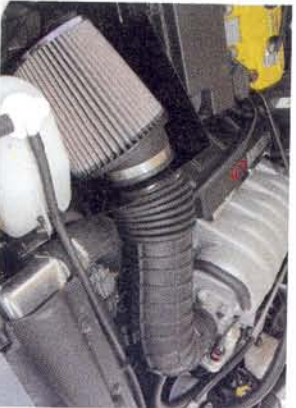
▲ Burnsville builds the air intake for the Hemi swaps. It comes as part of the company's installation kits and includes a K&N air filter.
