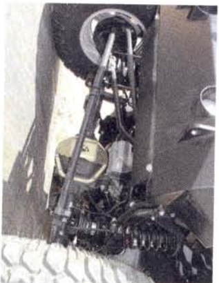
▲ Both Jeeps keep the stock drag link and the rod up front, the Wrangler Unlimited has Superfor 4.88 gears in addition to the stock electric lockers. It also has a Superlift diff guard, Superlift adjustable track bar, Superlift coils, and Walker Evans adjustable reservoir shock absorbers. The Rubicons have a sway bar that can be disconnected electronically, so you don't need quick-disconnect sway-bar links.
