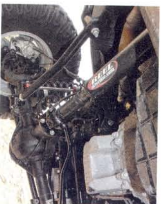
▲ Daystar JK arms are adjustable so we can adjust for caster and lift height. J.E. Reel CV driveshafts are strong and perfectly balanced. There are no driveline vibrations in either Jeep. The front Dana 44 on the JK is reverse-cut with the pinion up high out of harm's way. The front 44s have 30-spline inner axles, but 32-spline outers with big U-joints. Burnsville had the axles machined so full-circle C-clips could be used. The only problem with the JK is that the half-circle C-clips work their way out, letting the U-joint cap fall out. With the U-joint rattling around in the ears, the axle breaks. We had no problems at all with our 37-inch tires on the stock axles with the full-circle clips.
