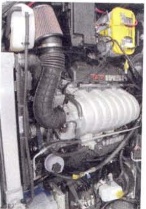
▲ The SRT 6.1 Hemi is a hand-built, balanced and blueprinted V8 with 425 hp in stock trim. It looks tight in the JK engine compartment but really is hardly wider than the stock 3.8 six it replaced. It's just longer. The big Howe aluminum radiator fits fine and, with the factory fan and shroud, keeps the 6.1 cool no matter what the outside temperatures are. We used Optima Yellowtop batteries in both Wranglers.
